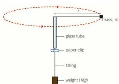
Circular motion can be investigated experimentally by tying a bung, with mass  $m$ , to a piece of string, and threading it through a glass tube. The other end of the string has a weight, with mass  $M$ , suspended from it. This provides the centripetal force,  $F = Mg$ , as the tension throughout the string is constant. The string is whirled in a circle, and the time taken for a complete rotation is recorded. The mass of the weight is altered and the experiment repeated.
